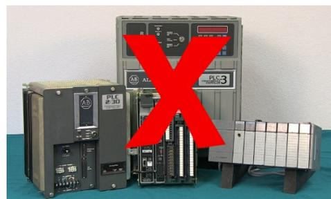
market inventory of A-B I/O equipment. Upgrades are most often desired due to limitations of the PLC CPU or programming software incompatibility with modern computers/Windows operating systems - not because the I/O is failing.
