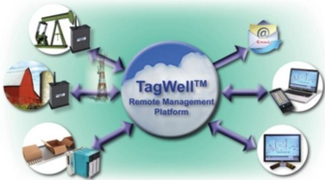
*SoftPLC Gateways can provide access to other control systems via SoftPLC's TagWell Cloud Remote Management Platform, and via direct modem connections acting as a remote access switch and/or as a data concentrator.*
