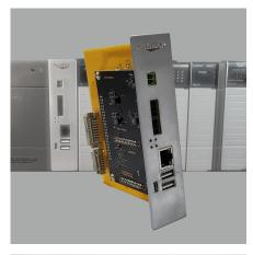
2. Replace the SLC-500 processor with a 1747-ASB remote I/O adapter. Connect your Smart or NeoPAC SoftPLC to the I/O adapter via "blue hose". SoftPLC Corp provides gently used 1747-ASB modules with 1 year warranty as our Catalog Number ICO-1747ASBKIT.
