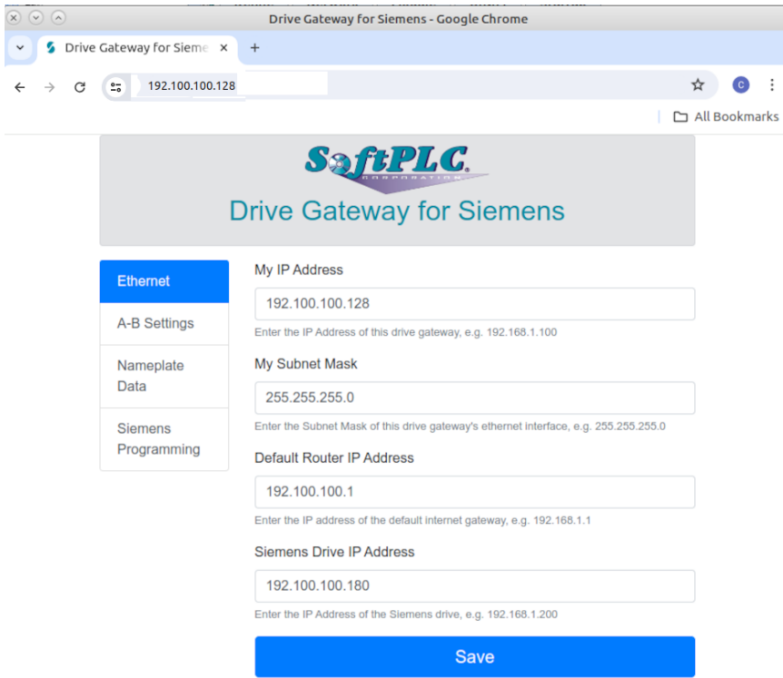
Figure 2. Siemens Drive Gateway Ethernet Settings
