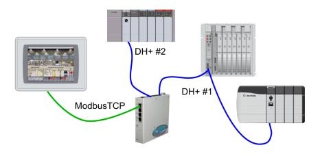
• Add I/O from another vendor to a PAC/PLC installation (*eg: ModbusTCP I/O such as Tealware, DeviceNet/Profibus, Modbus serial.*)
