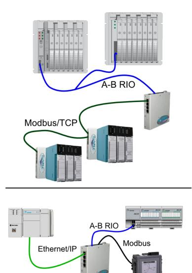
• Low cost serial to ethernet gateways (eg: Modbus to Ethernet/IP or ModbusTCP, DF1 to Ethernet/IP)
