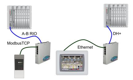
• Communicate data between devices on different network types.
