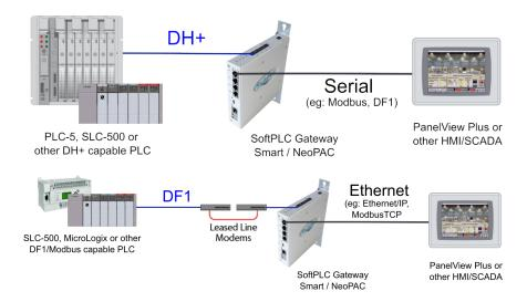
• Bridge devices between DF1 serial (or Modbus) and Ethernet networks (alternative to Allen-Bradley 1761-NET-ENI)
