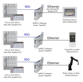
Upgrade HMI's, drives, or other devices on A-B Remote I/O networks without changing the A-B PLC logic or hardware!
