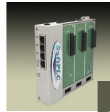
Smart SoftPLC/Adapter equipped with a Backplane3 interface
