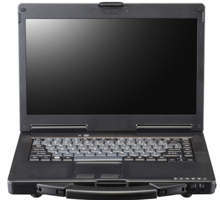
TOPDOC PLC-2 Programming Station (Cat No TD2-PS)
