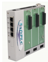
Smart SoftPLC w/ Backplane3 Interface (without and with modules installed)
