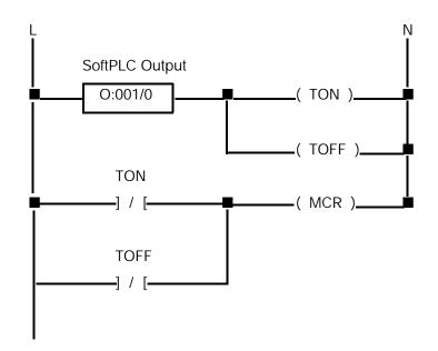
In the above ladder logic representation of the watchdog timer circuit, there are two timed relays, TON and TOFF. TON starts timing on the positive going edge (FALSE to TRUE transition) of the output bit (in this example 0:001/0 although any digital output can be used). Similarly, TOFF starts timing on the negative going edge (TRUE to FALSE transition) of the output bit.
